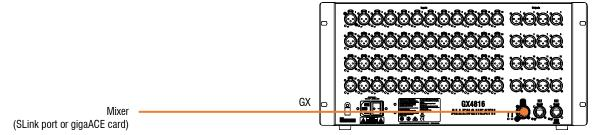
Switch on the mixer first, then the GX Expander. The GX port Lnk/Err indicators flash at a steady rate when the link is established. The red error indicator lights if a communication error is detected.
